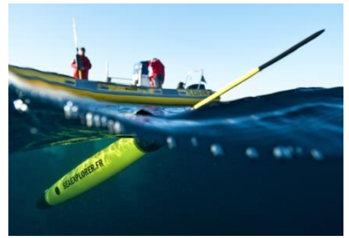
Deploying and recovering the glider from small boat
