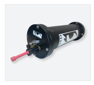
The Mini-T-SURVEY multiplexer is a dedicated fibre optic multiplexer system for oceanographic survey applications offering digital fibre optic transmission of multiple highspeed Ethernet and serial data channels over a single fibre optic link.
