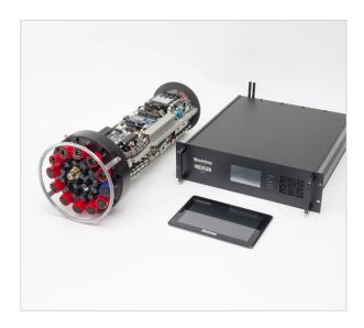
The MacArtney NEXUS MK VII is an advanced and versatile HD video, standard video, Ethernet, serial and multibeam sonar multiplexer based on Focal 907 telemetric technology. Providing a highly efficent link between surface and seabed, the NEXUS MK VII carries all signals over one single mode optical fibre via CWDM (coarse wavelength division multiplexing).
